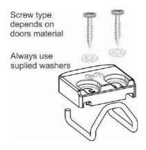
Due to the use of different door thickness and materials, the manufacturer has decided to leave the choice of screws to the installer. While installing, we recommend the showed assembly procedure of the strike.
