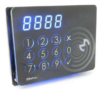
Metra Display ISO is a user interface device for Metra electronic locking systems. It reads ISO 15693, ISO 14443A, ISO 14443B and Mifare compatible RFID media as locker keys and displays the locker number on a four digit LED display. Integrated 12 key washable keypad enables additional user interaction (PIN code, locker number, etc.) and can be used for locking / unlocking instead of RFID media. It also signals a locker brake-in alarm.
