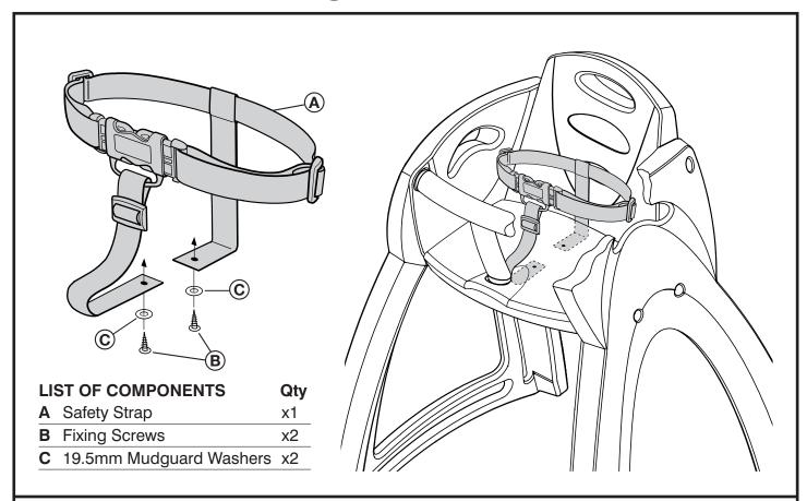
Invert chair, remove old Strap, & note fixing points (1) & (2) on base of Seat as (shown right).
