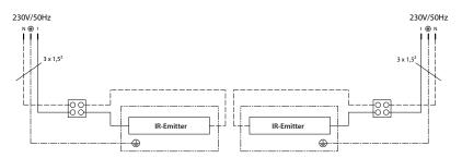
Note: Please bear in mind that each IR heater consists of two sections and has two connection cables.
